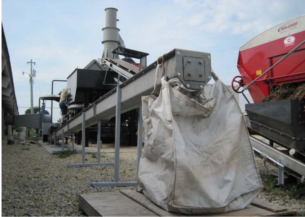
The ash auger fills a super sack to minimize handling.
